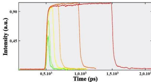
Fig. 2. Temporal pulse profiles measured between 35 ps and 1 ns with a fast response photodiode
