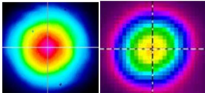
Fig. 4 Spatial profile at 1064 nm, 16 W (left) and 1550 nm, 10 W (right)
