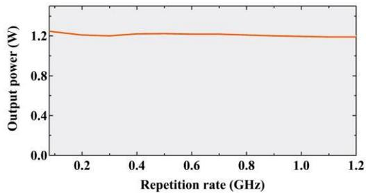
Fig. 3. Output power vs repetition rate measured at 15 different repetition rates
