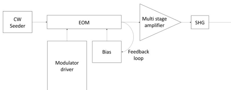
Fig. 1 Diagram of the laser system; CW, continuous wave; EOM, electro-optics modulator; SHG, second harmonic generator
